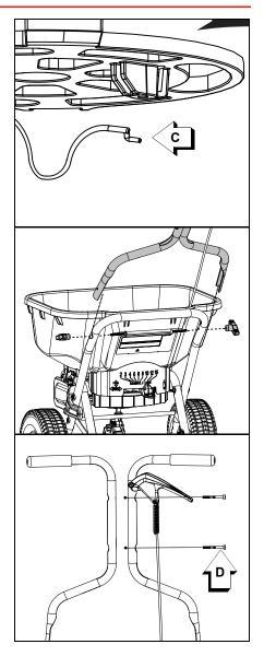
Remove upper handle bracket from lower handle bracket.
