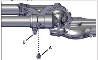
2. Remove the cutting head assembly.
