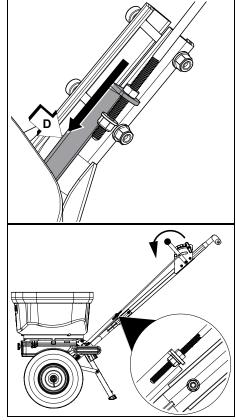
5. Position gate control lever fully forward, and tighten control rod nut and flange nut as shown.
