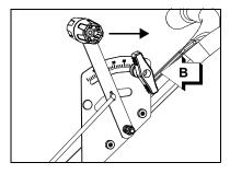
Push gate control lever (A) fully forward to close gate. Fill hopper with product. Fill hopper in an area that won't be damaged by spilled product.
