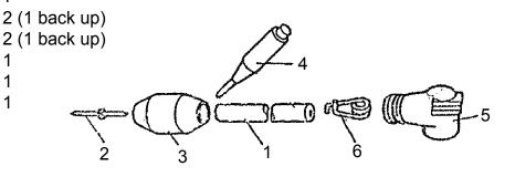
1. Cut away the damaged part of spark plug wire (1). Clean spark plug wire (1) and connector cover (3) with alcohol to insure a tight connection. Otherwise an electrical leak could develop.
