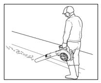
wide open throttle for at least 5 minutes every hour, and inspect/clean the spark arrestor screen after approximately 40 hours of operation.
