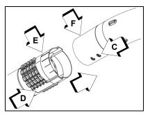
loosen pipe connections. Exclusive positive locking system allows pipes to be tightened. If loosening occurs, remove straight pipe, and reinstall according to instructions 3 and 4.
