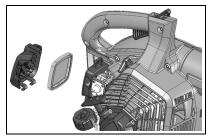
brush debris from filter. Replace filter if it is damaged, fuel soaked, very dirty, or the rubber sealing edges are deformed. Clean the filter with a neutral detergent. Do not use solvents for cleaning.
